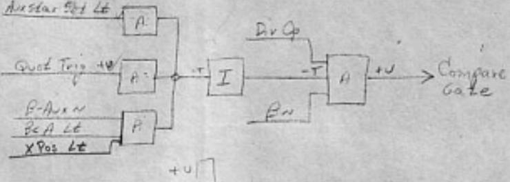
25. Set Sign Gate =  $(End\_{Div}\_{Lt})(Set\_{Quot}\_{Trig}) + (Set\_{Prod}\_{Sign}\_{Lt})(B\_{Aux}\_{Cycle})$
