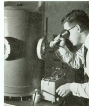
Scientist checks temperature as arsenic vapor diffuses into germanium, creating 4/100,000 -in. layer.
